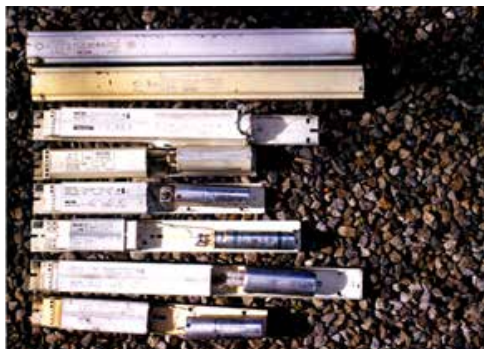
Fig. 1b: Capacitive ballast units from Knobel, Ennenda. The same devices as in Fig. 1a after the removal of the capacitor cover. Length (top appliance) = 40.7 cm
