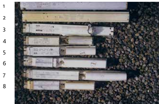
Fig. 1a: Capacitive ballast units from Knobel, Ennenda.
